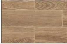
T-1 Distr: Virgina Tile Manufacturer: Virgina Tile Contact: Natasha Caitlyn 216.749.4540 Collection: Domestic Collection Wood Look Product #: VDC BLRB Finish: Matte Size: 8" x 40" Install: Horizontal running bond Grout Size: 3/16" Grout & Grout Color: TruColor by Bostik Jamoca H162
