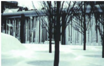
YORKVILLE PARK - TORONTO, CANADA, 1994 This fountain incorporates heated drip lines that feed stainless steel cables to form a rain curtain in the summer and an icicle sculpture in the winter.
